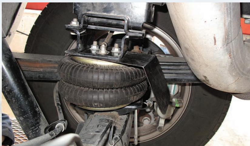
The upper air bag support bolts securely to the frame. The air spring suspension brackets are preassembled before locating them on top of the axle. A heat shield protects the air bags from the exhaust. Mounting brackets have been beefed up to handle the heavier loads.
