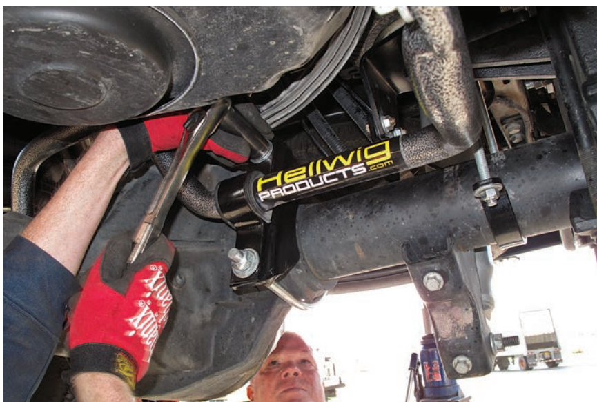
(Top) We replaced the factory front sway bar with a Hellwig Big Wig Sway Bar. The OEM end links were reused, but the New Hellwig brackets use fresh polyurethane bushings. (Bottom) The Hellwig Big Wig Adjustable Sway Bar on the rear was an easy bolt on. Small spacers in the kit (seen in the photo) helped accommodate the truck's pre-existing Rancho 4-inch lift kit.
