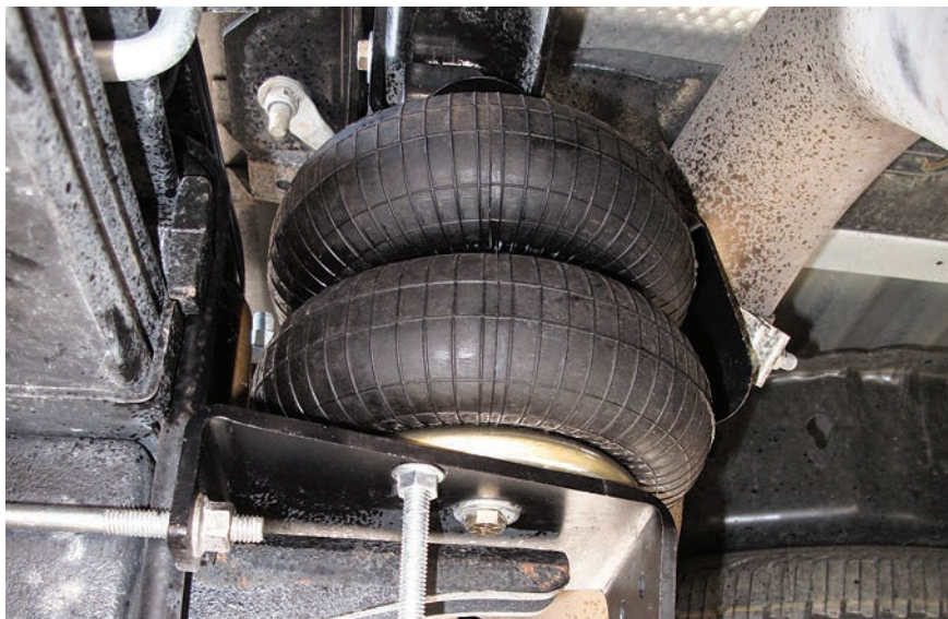
Contitech, a division of Continental Tire in Germany, makes the Hellwig air bag springs. A unique cantilever bracket supports the air bag on the rear bump stop. The top air bag bracket bolts through the frame, and a U-bolt clamps the cantilever bracket in place.
