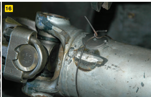
14) Any slight out-of-trueness is corrected with a quick blast from a torch. 15) Setting up the high-speed precision Axiline balancing machine developed by Drive Line Service of Sacramento is initially done with the experienced hand of the technician. He can feel the slightest vibration. 16) Small, flat washer-size weights are temporarily placed and moved to obtain the perfect balance. They are then welded into place.
