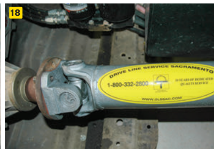
17) Some of the special sockets and wrenches needed to remove or install driveshafts may not be in most toolboxes. Check before you start. 18) The simple U-joint could be the weak link in today’s powerful drivetrains. Have you checked yours? 19, 20) The expert mechanics at Ken Imler Diesel Performance installed the overhauled driveshafts and kept an eye out for any other problems.
