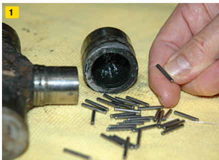
1) These little needle bearings are what connect your vehicle's engine to the tires on the ground. 2) Time and miles had taken their toll on the stub shaft splines. 3) The blue glide coat on the new Spicer shafts extended farther up the splines for reduced wear.
