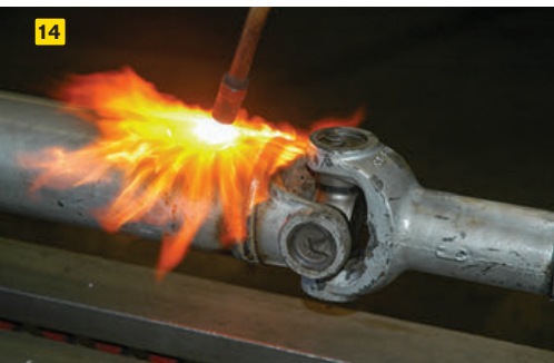
14) Any slight out-of-trueness is corrected with a quick blast from a torch. 15) Setting up the high-speed precision Axiline balancing machine developed by Drive Line Service of Sacramento is initially done with the experienced hand of the technician. He can feel the slightest vibration. 16) Small, flat washer-size weights are temporarily placed and moved to obtain the perfect balance. They are then welded into place.
