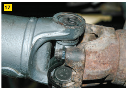
17) Some of the special sockets and wrenches needed to remove or install driveshafts may not be in most toolboxes. Check before you start. 18) The simple U-joint could be the weak link in today’s powerful drivetrains. Have you checked yours? 19, 20) The expert mechanics at Ken Imler Diesel Performance installed the overhauled driveshafts and kept an eye out for any other problems.
