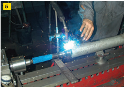
4) The process of cutting off the worn driveshaft yokes and stub shafts was accomplished using a lathe. 5) Once the stub shaft was precisely aligned in the driveshaft, it was welded in place and rechecked. The goal was to keep a tolerance of .003 of an inch. We got ours down to .001. 6) As with other driveline components, rebuilding a CV joint is a job for an experienced technician.
