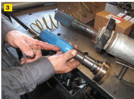
1) These little needle bearings are what connect your vehicle's engine to the tires on the ground. 2) Time and miles had taken their toll on the stub shaft splines. 3) The blue glide coat on the new Spicer shafts extended farther up the splines for reduced wear.
