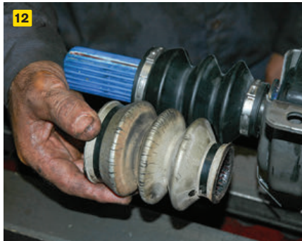
10, 11) The carrier bearing supports the midship driveshaft where it joins the rear driveshaft with its splined stub shaft. It is bolted to a frame cross member. 12) A new dust boot protects the midship driveshaft splines where it mates with the rear driveshaft. 13) After pressing the new yokes into the shafts, the seam is welded and then rechecked for trueness.
