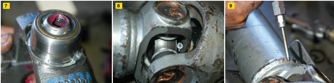
7) Inside the ball of the CV joint, the small needle bearings must be perfectly in place before reassembling. 8) Maintenance people often overlook the lube fitting on the CV joint. 9) To properly lube the CV joint, a needle attachment on the lube gun is required.
