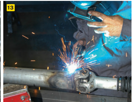
10, 11) The carrier bearing supports the midship driveshaft where it joins the rear driveshaft with its splined stub shaft. It is bolted to a frame cross member. 12) A new dust boot protects the midship driveshaft splines where it mates with the rear driveshaft. 13) After pressing the new yokes into the shafts, the seam is welded and then rechecked for trueness.
