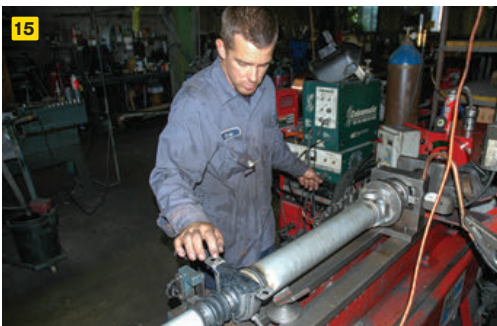
14) Any slight out-of-trueness is corrected with a quick blast from a torch. 15) Setting up the high-speed precision Axiline balancing machine developed by Drive Line Service of Sacramento is initially done with the experienced hand of the technician. He can feel the slightest vibration. 16) Small, flat washer-size weights are temporarily placed and moved to obtain the perfect balance. They are then welded into place.
